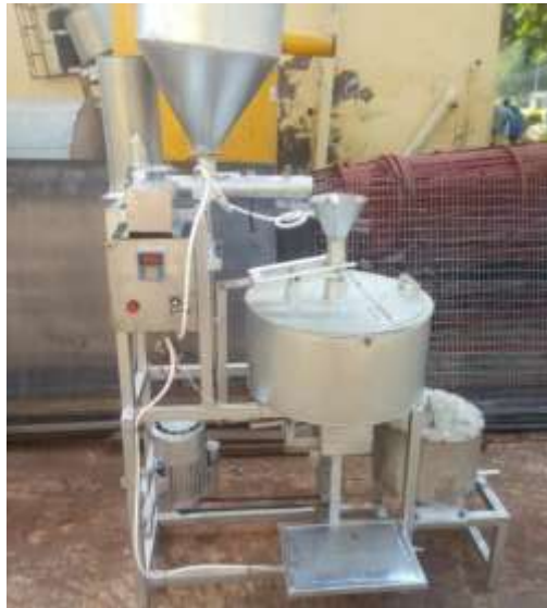
Figure 4. Plate II: The developed improved automated grain drinks processing machine
